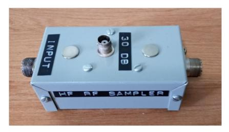
The construction was the same as his except I used RG58 coax for the inner conductor and used a T50-2 core because that is what I had.
